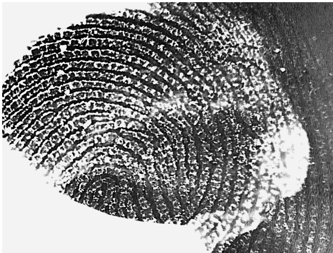
FIG. 5—Photograph of fingerprint on sticky side of black plastic electrical tape directly developed by staining with CdS nanocrystals.
